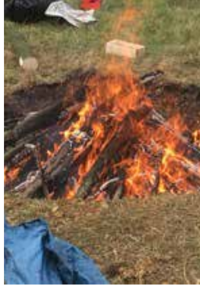
After the fire had propagated throughout the fuel, a charge with larger diameter wood was added and allowed to burn, generating a significant amount of embers
