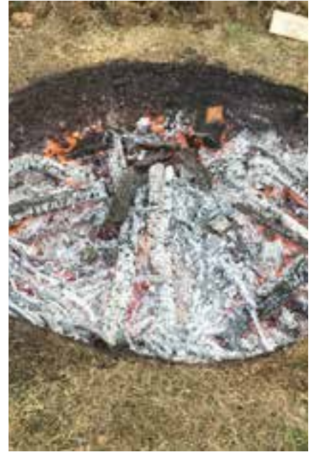
Last wood added, 1 hr 5m after ignition - more wood was added wherever we could see pots poking through the ash, trying to keep them covered
