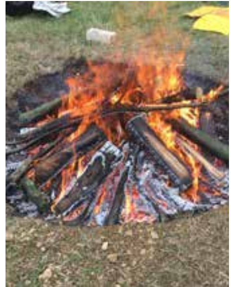
After the fire had propagated throughout the fuel, a charge with larger diameter wood was added and allowed to burn, generating a significant amount of embers
